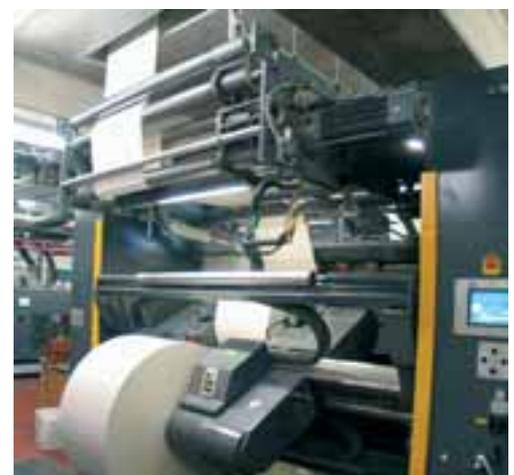
The 9300 Servo PLC product range and Winder technology package are the key to achieving complete winding, including control of the winding calculator with precise pilot control of the torque and speed according to how full the reel is. Also the traverse control is supported by the drive's software.
